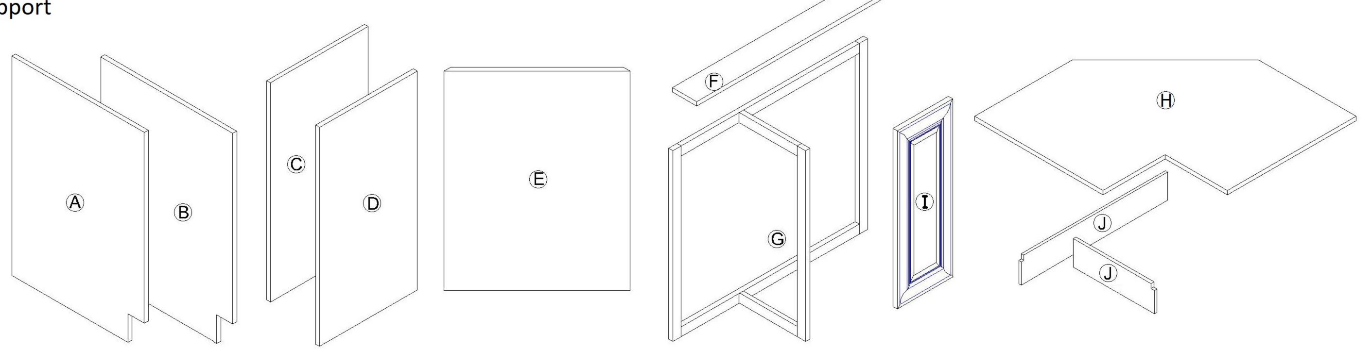
\* Face Frame G Need To Be Inserted To The Bottom Panel Before Attacking Side And Back Panel
